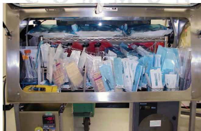
Figure 3: Transfer isolator fully packed with components (23-ft 3 316 SS transfer isolator with 3 gloves, 2 circulation fans, high-efficiency particulate air filters, and a pressure blower). Cycle time is 83 min.
