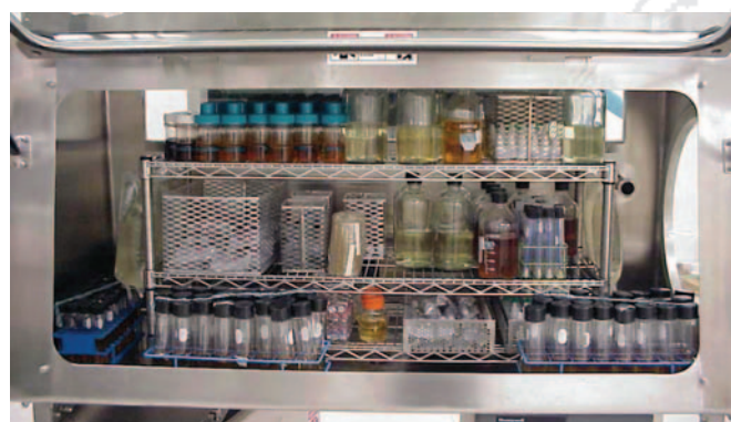
Figure 2: Transfer isolator fully packed with media (23-ft 3 316 SS transfer isolator with 3 gloves, 2 circulation fans, high-efficiency particulate air filters, and a pressure blower). Cycle time is 83 min.
